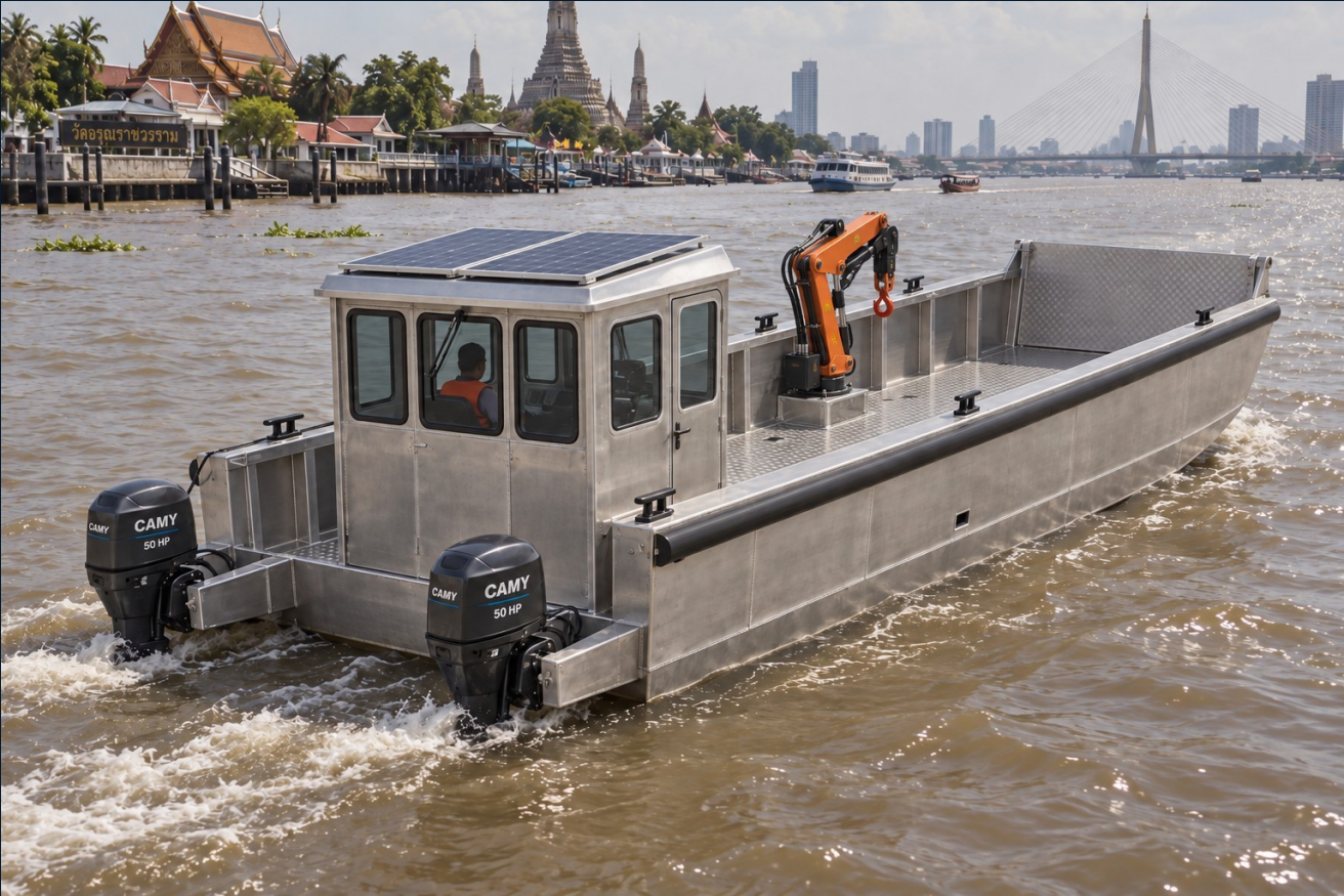
Concept image. Confirmed motor rating: 50 kW per unit.
